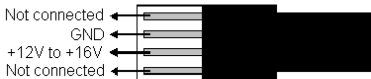
FIG. 1-6 MOLEX CONNECTOR PIN-OUT IN BT VERSION
