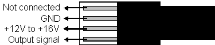
FIG. 1-4 MOLEX CONNECTOR PIN-OUT IN MT VERSION
