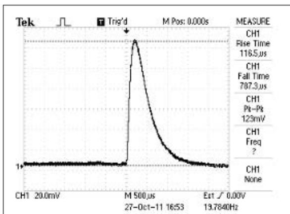
**Figure 1:** Typical voltage output for QE8SP-B-BL Joulemeter
