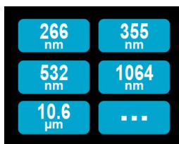
Figure 3 The 6 wavelength buttons can be customized by the user
